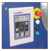
As a modern machine, the Bandum SH/S is PLC controlled. The operator interface is a highly intuitive, icon driven, touch screen display. This allows to quickly change the basic settings of the machine by selecting one of the of pre-defined 'recipes'.
